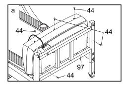
With the help of a second person, carefully raise the Upright Base (97) as shown. Carefully pivot the Hood (123) off.
